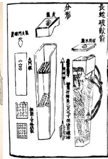
A depiction of the 13th Century "long serpent" rocket launcher. The holes in the frame are designed to keep the rockets separate, from the 1510 edition of Wujing Zongyao .
